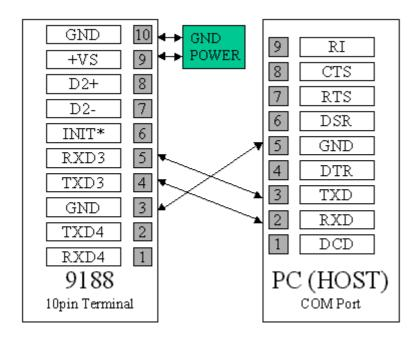
Connect COM3 to DTE. Wiring diagram:
