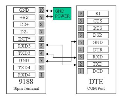
The 9188 library functions can be used to control COM3. "InstallCom3{}" is used to initialize the baud rate of the format of COM3. An interrupt driven driver will be loaded and 1KB of queue buffer is given. "ToCom(3,data)" can be used to send data to COM port. Use "IsCom(3)" to know if there is any data received and "ReadCom(3)" can get the first data from queue.
