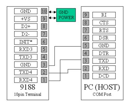
Use Hyper Terminal program under Windows 9X or 2000. After 9188 is powered on, a command prompt will be shown in the window of hyper terminal.
