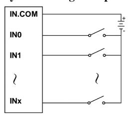
TTL/CMOS signal Input
